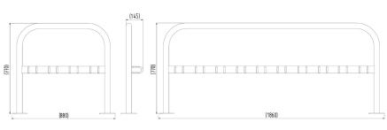
The Kids Scooter Rack is ideal for the storage of kids scooters while they are at school. The Rack is available in single or double sided with hoops welded to the cross bar that allow the scooter to be secured with a cycle lock.
