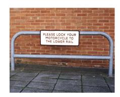
The Motorcycle Security Barrier is ideal for securing motorcycles. The Security Barrier is based upon a standard perimeter barrier of 76mm outside diameter tube, but has the addition of loose steel bars inserted into the lower horizontal tube and legs, this greatly increases the difficulty of cutting through the tube in order to make away with anything locked to the barrier. The Motorcycle Security Barrier is fully galvanised and only available in a Concrete in finish.
