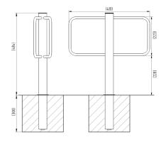
Part Number 138 200 007 138 200 049 Description Model SU (V) - Concrete In Model SU (V) - Bolt Down <u>Weight (kg)</u> 5kg 5kg
