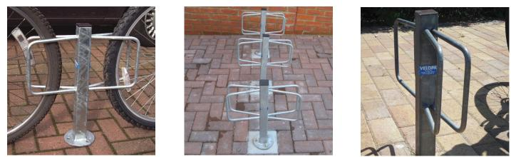
The SU (V) is a freestanding variant of the simplest cycle holder, the Model R. A familiar sight throughout the UK, these holders allow the tyre of the bicycle to be supported. The Model SU (V) is a suitable for two bicycles. The stand is fixed to the ground, in either concrete in or bolting down versions and can be spaced at 610mm apart for cost effective cycle parking.
