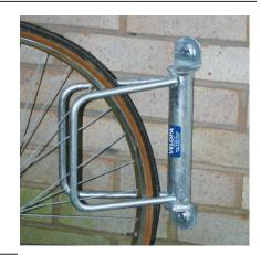
The simplest cycle holder, a familiar sight throughout the UK, allows the tyre of the bicycle to be supported. The stand is fixed to a suitable wall and can be spaced at no less than 610mm between holders for cost effective cycle parking. The Model R is available in either 90° or 45° versions which allow for cycles to be parked either head-on or angled.
