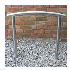
The Harlestone Cycle Stand is a shaped tubular cycle stand. The design allows the frame of the bicycle to be secured by the users own security lock. The Harlestone Cycle Stand is suitable for securing two bicycles. The Harlestone Cycle Stand is available in galvanised steel, Galvanised & Coated or Grade 304 Stainless Steel, with ragged feet for casting into new concrete or flanged feet for bolting to an existing surface.
