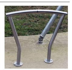
The Dallington Cycle Stand is a shaped tubular cycle stand. The design allows the frame of the bicycle to be secured by the users own security lock. The Dallington Cycle Stand is suitable for securing two bicycles. The Dallington Cycle Stand is available in galvanised steel, Grade 304 and Grade 316 Stainless Steel, with raggedfeet for casting into new concrete or flanged feet for bolting to an existing surface.
