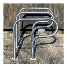
The Rugby Cycle Stand is a P shaped tubular stand, designed to provide cyclists with a secure stand for locking their cycles. The design allows the frame of the bicycle to be secured by the users own security lock. Suitable for securing two bicycles. The Rugby Cycle Stand is available in both galvanised and stainless steel, with ragged feet for casting into new concrete or flanged feet for bolting to an existing surface.
