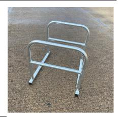
The Bilton Cycle Toastrack is a floor fixed cycle rack based upon the Bilton Cycle Stand. The Bilton Cycle Toastrack consists of Bilton Cycle Stands welded at 800mm centres to floor fixed box section rails. The benefits of a Cycle Toastrack over individual stands are reduced installation costs and pre-determined gaps between stands, each stand is suitable for parking two bicycles. The Bilton Toastrack is ideal where cycle parking in large numbers is required.
