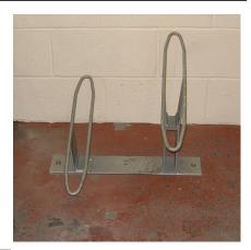
The Type H Cycle Rack is floor fixed cycle rack designed to hold the front wheel of the cycle off the ground. The Type H Cycle Rack is available as a 2 bicycle holder with cycle parking centres at 350mm. Each holder allows the user to lock their cycle through the front wheel to the stand.
