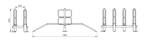
The Type E Cycle Rack is a floor mounted cycle rack based upon the Model R Holder. The Type E offers a high cycle parking density with cycle stands on two sides, the alternating high and low holders allow for high cycle parking density of 305mm between stands.
