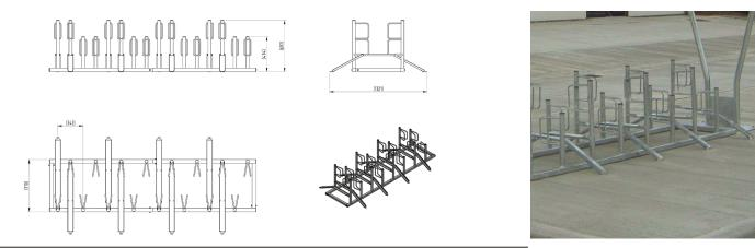
The Type A Cycle Rack is a floor mounted cycle rack based upon the Model R Holder. The Type A offers an extremely high double sided cycle parking density. The High and Low holders combined ensure that cycles are parked only 170mm apart (typical parking distance for a Sheffield Cycle Stand is 500mm). The high Holders, which incorporate Ramps are arranged in opposite facing pairs, as are the low holders, this combination ensures that all holders can accomdate bicycles at the same time.
