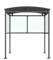
The Blencoe shelter is a free-standing, open fronted shelter designed for on site assembly, constructed from galvanised mild steel. Complete with a 1mm galvanised sheet roof, and 4mm PETG clear sheet ½ side panels. Side-to side curved roof.
