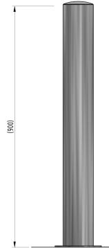
The galvanised mild steel range of 900mm tall fixed bollards are suitable for a range of applications and are ideal as a complement to the Autopa ranges of Parking Posts, RemovaPosts and RetractaPosts.
