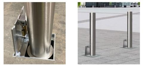
The Removable Bollard offers an effective, simple and robust way to protect premises and vehicles. Removable Bollards are particularly suitable for locations where occasional access is required, the simple tab and padlock system provides an easy to operate solution for locking the bollard in place. The Stainless Steel Removable Bollard is 750mm above ground and is available in a range of outside tube diameter sizes from 48mm through to 204mm. Padlock to secure is available at an extra cost.
