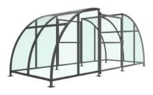
The SCC1 is a variant of the Stratford Compound, and is a free-standing shelter with a Mesh Door lockable by padlock (not included) designed for on site assembly. Constructed from galvanised mild steel, complete with a 4mm PETG clear sheet curved roof and end panels.
